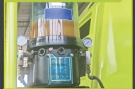
AUTOMATIC CENTRALIZED LUBRICATION SYSTEM
